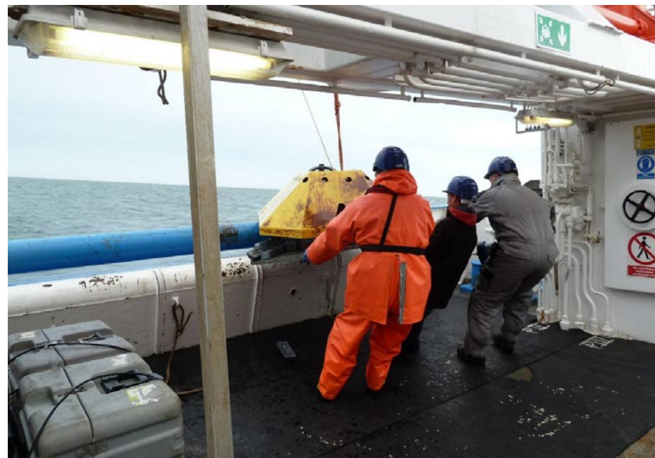
ADCP's Being Deployed
