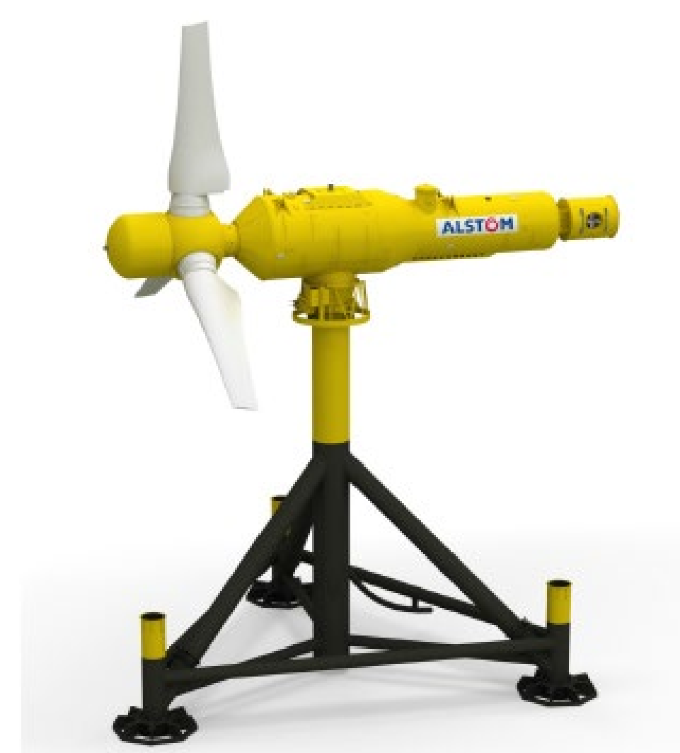
Single TEC, capable of rotating to face flow, on a tripod structure, pin piled into the seabed (copyright Alstom 2014)
