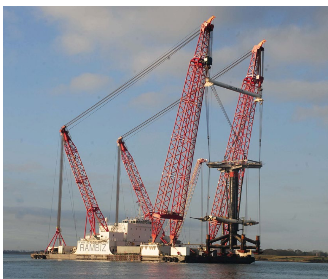
Heavy Lift Barge “Rambiz” installing SeaGen S foundation in Strangford Lough
